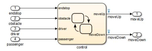
The referenced model implements controller logic with a Stateflow® chart.
