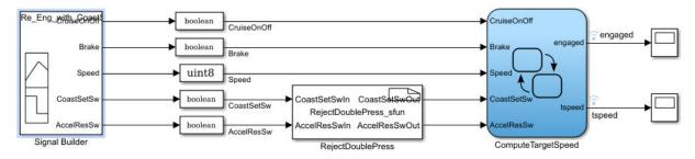
The model is a cruise control system that consists of test cases and input signals from a Signal Builder block. The signals from the Signal Builder act as inputs to the Stateflow chart ComputeTargetSpeed, which engages or disengages the cruise control system and sets the target speed, tspeed.
