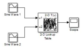
In this model, the lookup table indices are 1, 2,..., 10 in each direction. The Sine Wave 2 block is out of phase with the Sine Wave 1 block by pi/2 radians. This generates x and y numbers for the edge of a circle, which you see when you examine the resulting Lookup Table coverage.
